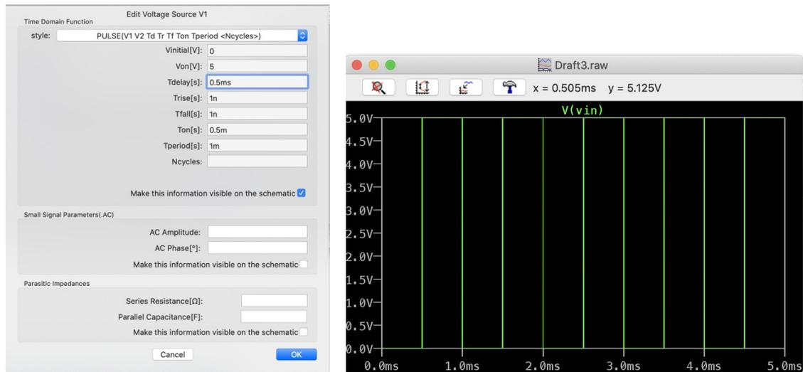
Figure.2 Screenshot to set up the 1kHz square wave, starting at 0V(low) and 5V (high)
